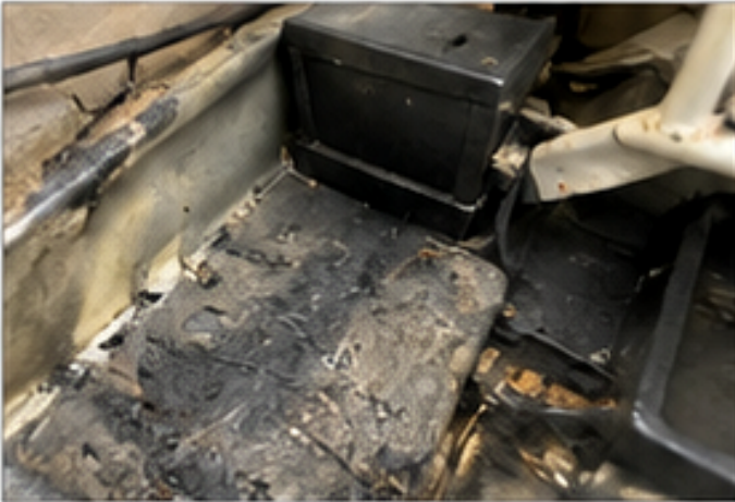
Thermal damage to cockpit floor around the battery box (viewed from above).
