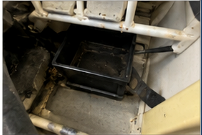
Battery box location between seats, under the right seat base.
